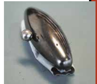
Set the ball on the magnet. It will move to the pole—the strongest part of the magnetic field. Make a loop of duct tape and stick it at 90 degrees from the pole. Have kids tape their magnets to the table so the pole is in the same plane as the rolling ball.
