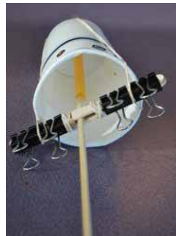
Kids can add binder clips to the plunger. When pulled back against the rubber bands, the added weight (i.e., mass) gives the plunger more potential energy, enabling it to do more work.
