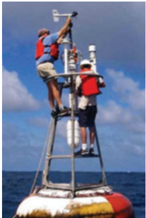
Remote Automated Weather Stations transmitting to GOES
