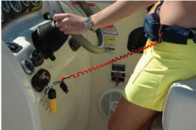
Hooked from the ignition to your life jacket, waist, wrist or thigh, this lanyard shuts off the engine and stops the boat if the operator is thrown overboard.
