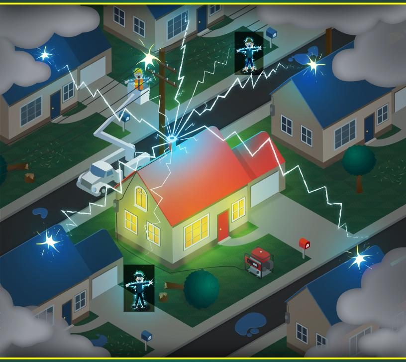
Transfer switches isolate utility power and generator power to prevent backfeeding, which can be deadly. Backfeed can follow wires and harm those nearby, including utility workers making repairs. Transfer switches also protect the home from electrical fires caused by short circuits and improper connections. Transfer switches should only be installed by a qualified electrician.
