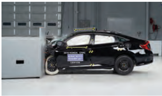
A 2016 Honda Civic undergoes a FRONTAL-CRASH TEST at the IIHS facility.
