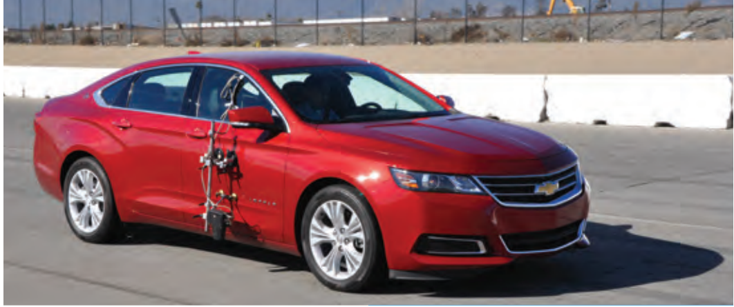
(Clockwise from top left) An OPTICAL FIFTH WHEEL is used in braking and acceleration tests at the Auto Club Speedway in Fontana, California; measuring a vehicle's TURNING CIRCLE ; using a DECIBEL METER to measure interior sound levels.
