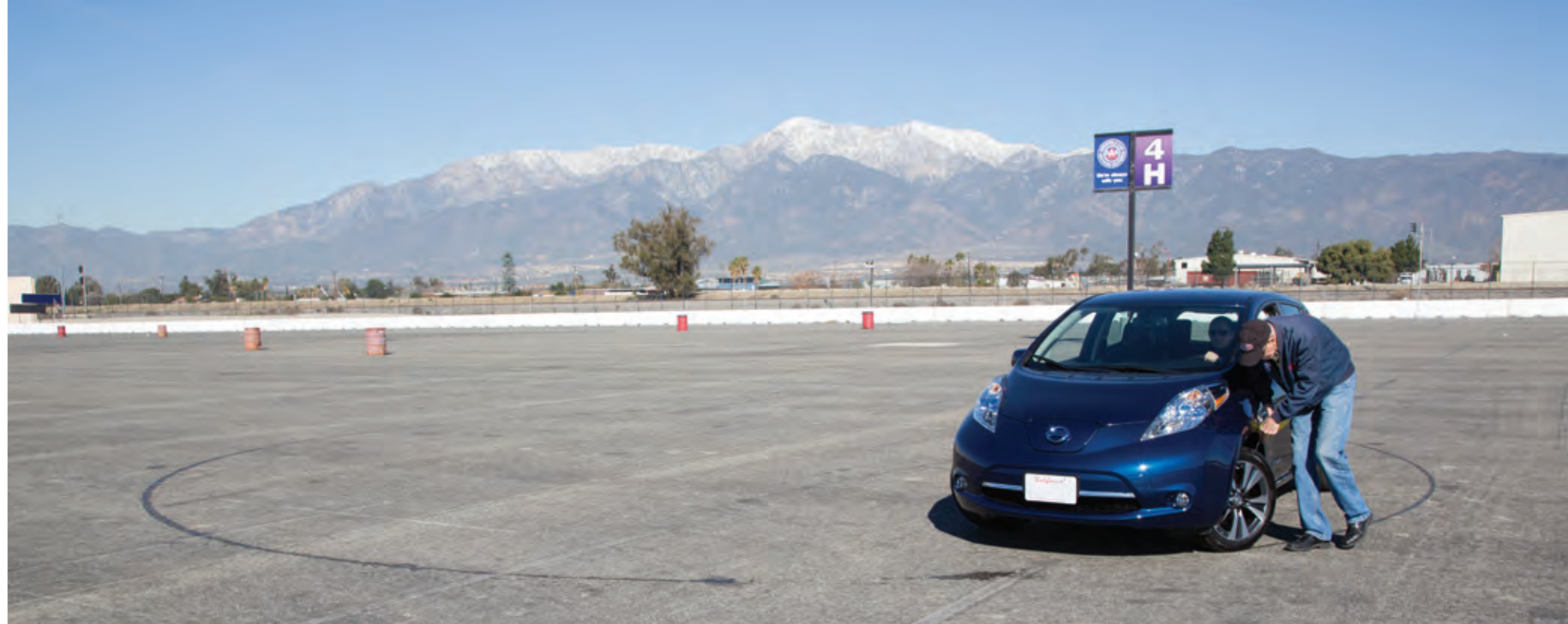
(Clockwise from top left) An OPTICAL FIFTH WHEEL is used in braking and acceleration tests at the Auto Club Speedway in Fontana, California; measuring a vehicle's TURNING CIRCLE ; using a DECIBEL METER to measure interior sound levels.
